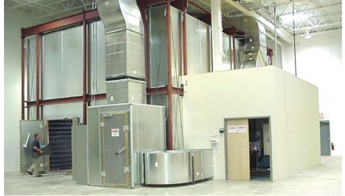
Large test chamber with auxiliary cooled shield room and noise controlled annex.
